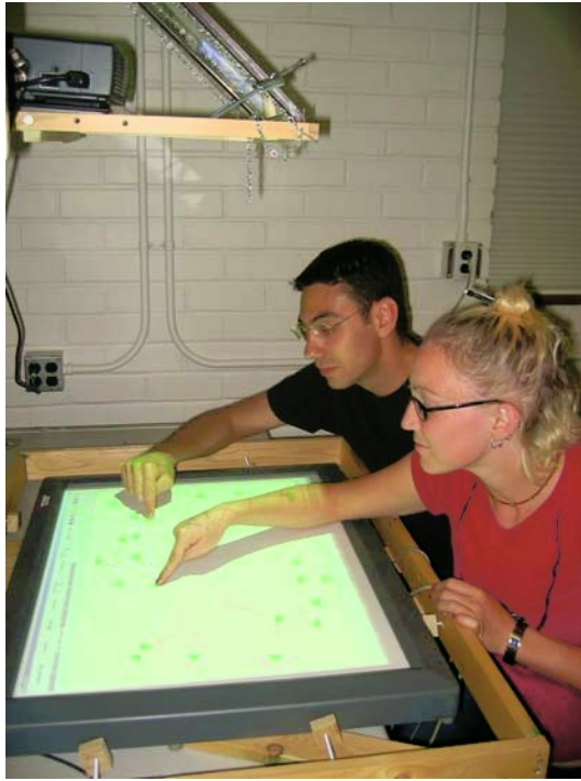
Fig. 2. Physical setup of the DiamondTouch table setup with two users untangling graphs.
